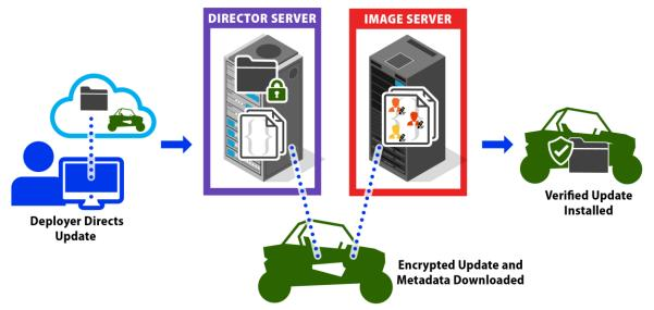
Figure 3. Update Deployment Process
