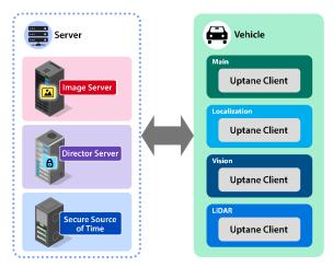
Figure 1. Server and Vehicle Architecture Depicting the Separation of Roles
