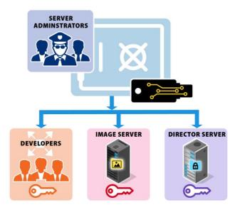
Figure 4. Key Hierarchy with Server Administrators Issuing and Validating Developer and Server Keys
